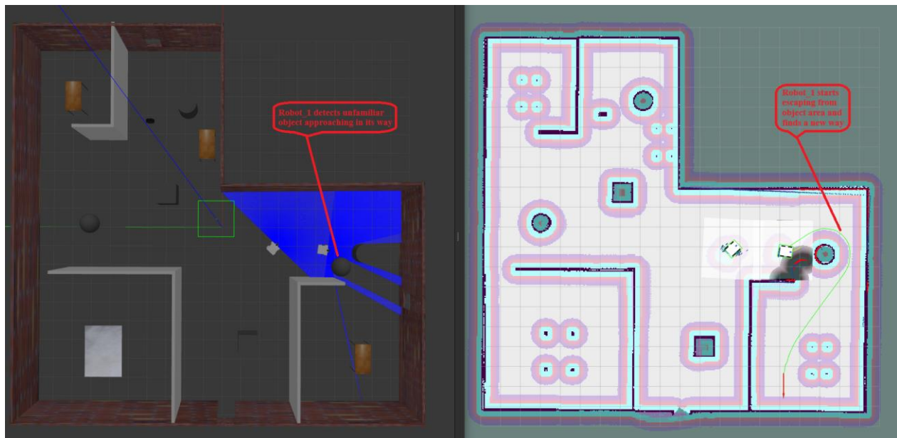
Figure 21(d). Robot_1 Object identification (the unfamiliar object that comes in its way).
