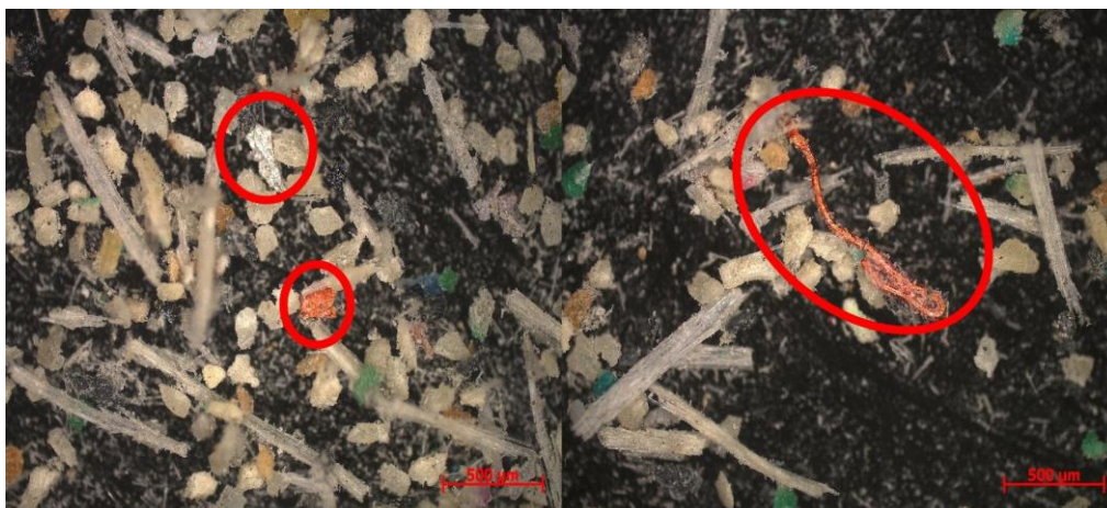
Figure 5. 4: Microscopic analysis of dry aggregates showing entrapment of metallic particles.
