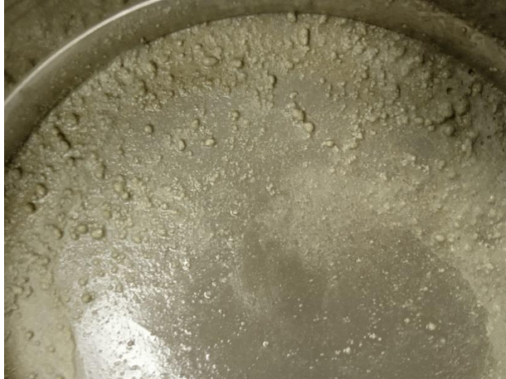
Figure C. 4: Particle aggregation during wet sieve analysis following intense agitation pretreatment at 500 rpm stirring speed.
