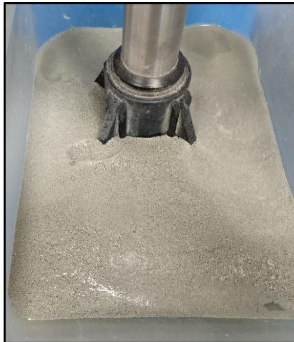
Figure 5. 7: Stable foam layer at the pulp-air interface formed solely by high-speed agitation at 2000 rpm (no aeration or frother addition).
