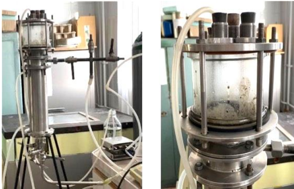
Figure 13 Fed-batch anaerobic bioreactor used during the experiments
