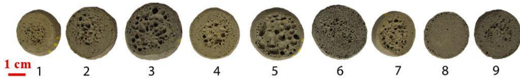
Figure 48. The pore structure of nine groups of specimens
