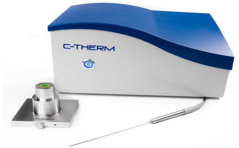
Figure 30. Thermal conductivity analyser instrument (C-Therm TCi)
