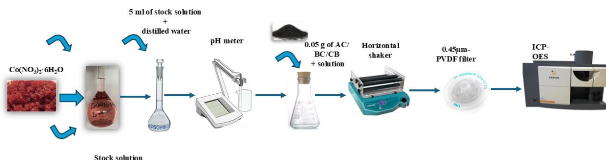
Figure 17. The workflow of the adsorption tests employed during the study
