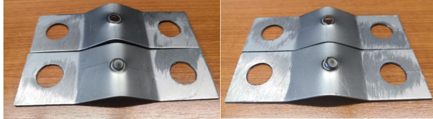
Figure 7.4. Plug failure mode in sample C1 is on the left and Plug failure mode in sample C12 is on the right in DP600 samples.
