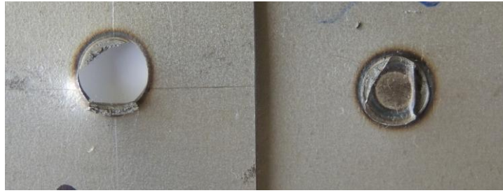
Figure 7.7. Partial plug failure mode in sample C4 of MS1400.
