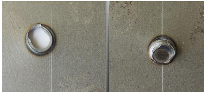
Figure 7.10. Partial plug failure mode in sample T4 of T-S test samples.
