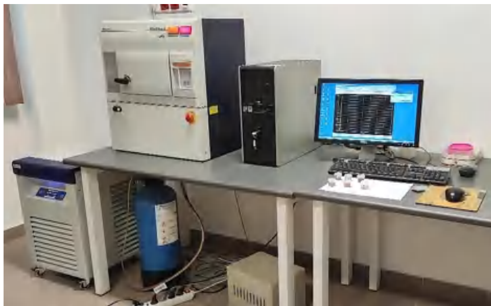
Figure 6. A Rigaku Miniflex II X-ray diffractometer setup in ceramic's laboratory at the University of Miskolc
