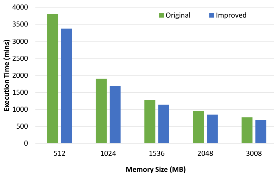
Figure 3.23: The makespan of the two algorithms with Inspiral (LIGO) workflow running on different Lambda memory sizes.
