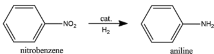
Figure 10 General reaction of nitrobenzene to aniline by hydrogenation
