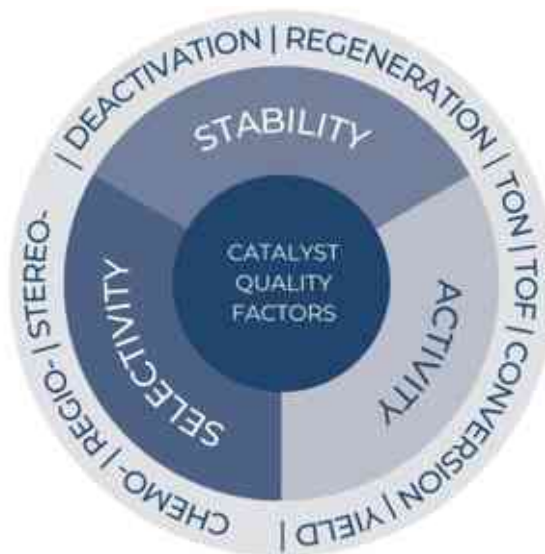
Figure 4 Most important catalyst qualification factors 15 (TON – Turnover Number, TOF- Turnover Frequency)
