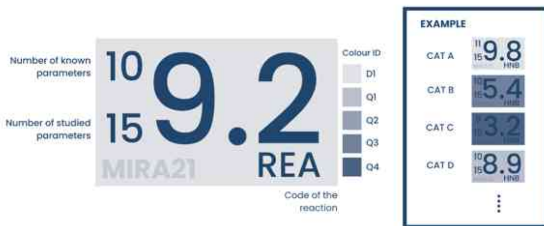
Figure 12 Visualization of quantitative description of a catalyst by MIRA21 number with corresponding classification and colour code: D1 (top10%), Q1(0-25%), Q2(25-50%), Q3(50-75%), Q4(75-100%), the deepening of the colour indicates the rank
