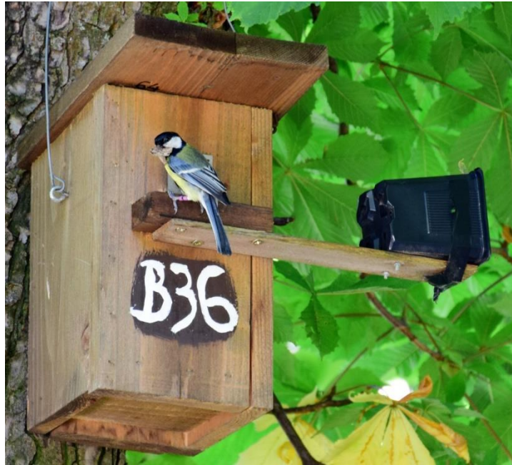
Figure II.3. Nest box design. We placed a wooden shelf in front of the entrance hole which allows the birds to pause for a moment. We attached a black plastic box for camouflaging the camera. Photo by Csenge Sinkovics, 2019.
