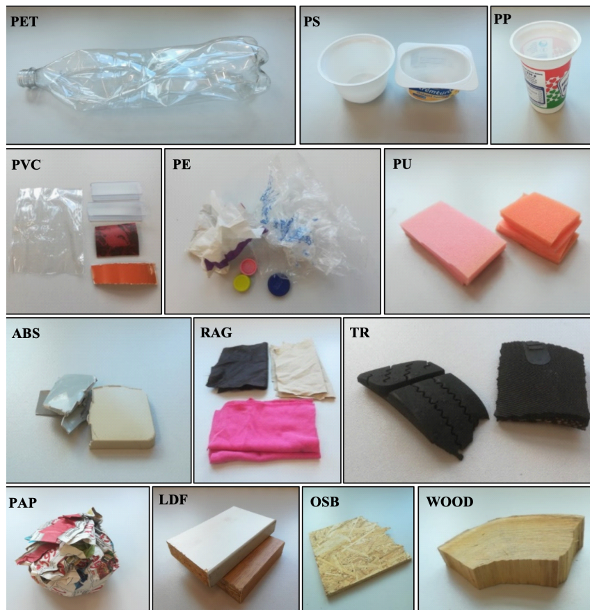
Figure 4. Solid-waste specimens for combustion tests
