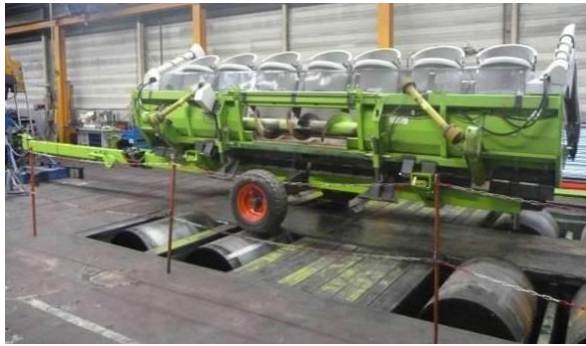
Figure 2.6: Measurements on roller test bench
