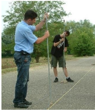
Figure 2.4: Profilometer in operation on an asphalt surface
