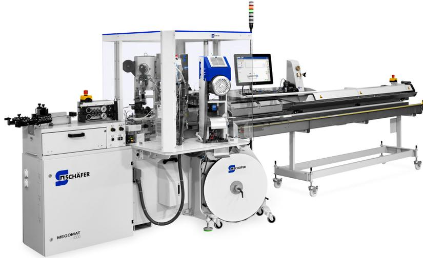
FIGURE 4.6: The studied automatic crimping machines log all the states and both setup and changeover activities.
