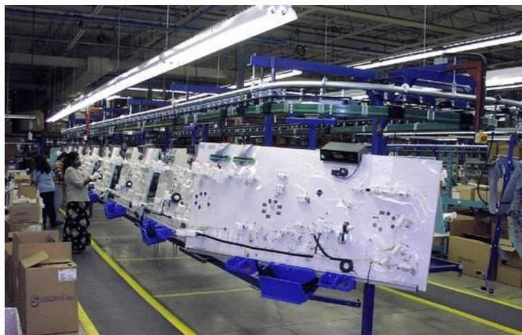
FIGURE 3.1: The wire harness paced assembly conveyor (often referred to as a rotary) contains assembly tables consisting of connector and clip fixtures [175].
