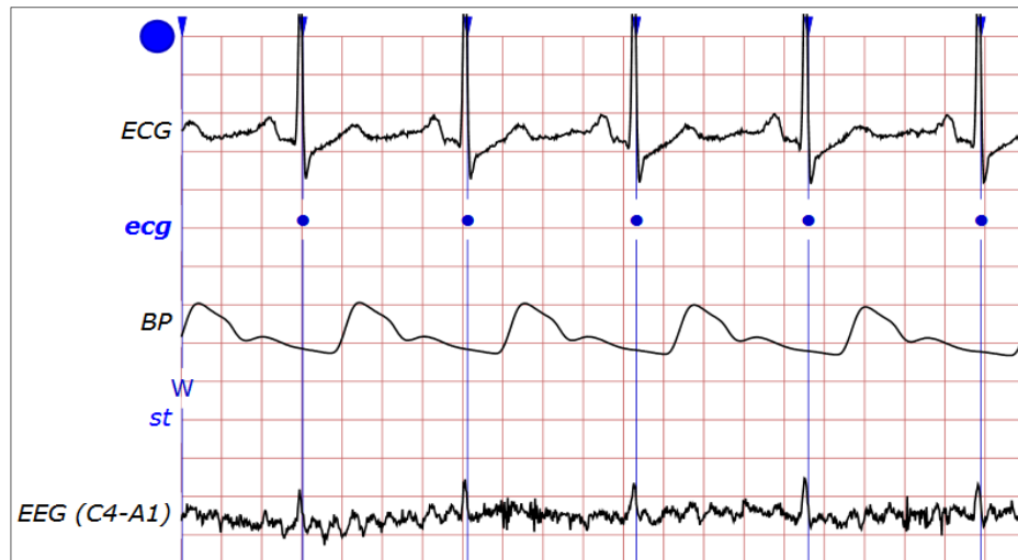
Figure 3-9: Annotated measurement from the MIT-BIH Polysomnographic database showing ECG, Blood Pressure and EEG signals. Note the pronounced ECG artifact contamination on the EEG channel (data record: https://physionet.org – slpdb/slp32 ).
