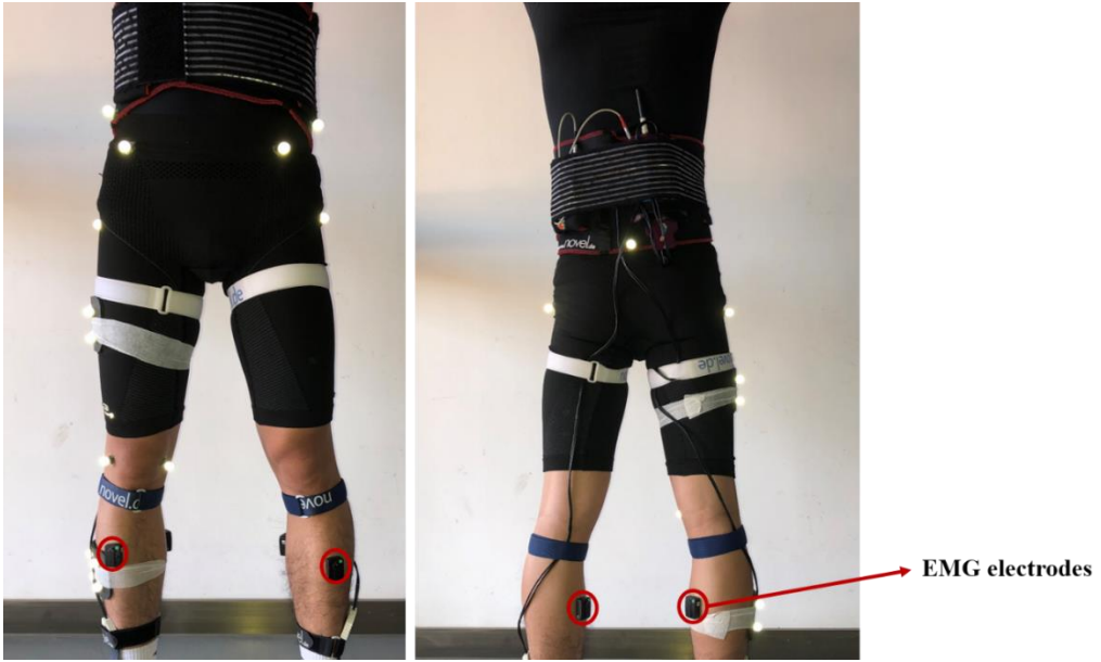
Figure 20 The placement of the EMG electrodes on the lower limbs.
