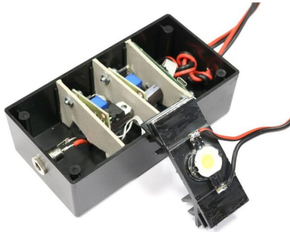
Figure 67. The photo of the pattern generator, LED drivers (in plastic enclosure), and the power LED.
