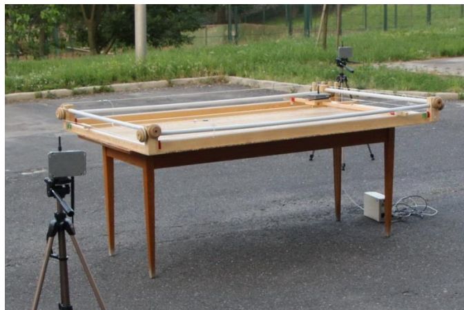
Figure 30. Radio-interferometric measurement devices (on tripods) and the plotter-like table used to move the tracked device.
