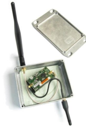
Figure 51. Dual-radio interferometric phase measurement device
