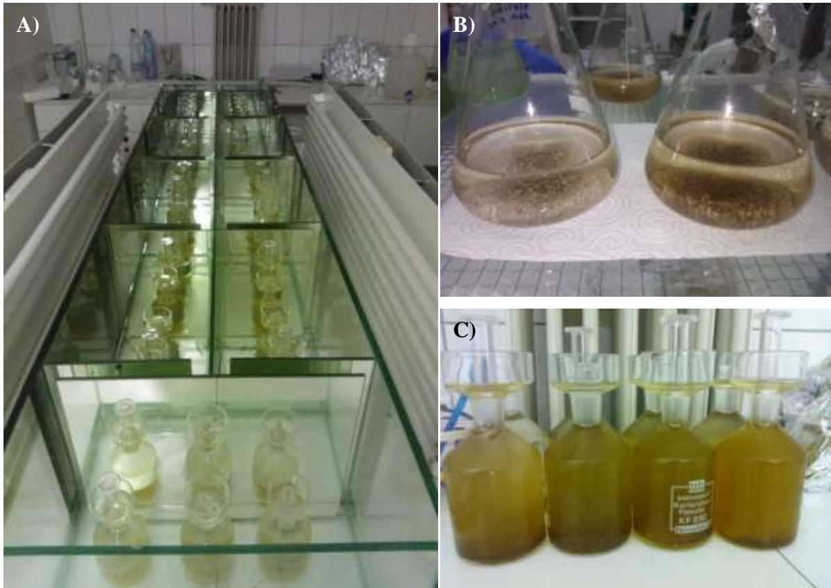
Fig. 5 The applied photosynthetron (A), the cultures (B) and the Karlsruhe flasks (C)
