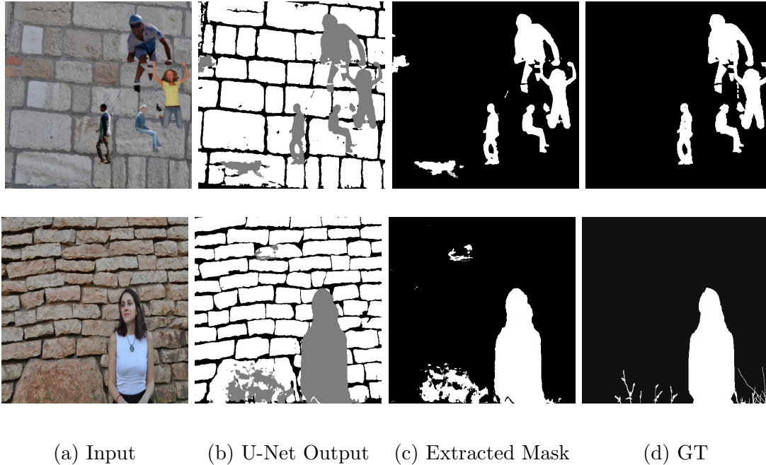
Figure 2.8: Pre-processing Stage results: (a) Input: wall image occluded by irregular objects (first row: synthetic occluding objects, second row: real occluding objects), (b) U-Net output with brick, mortar and occluded classes (c) automatically estimated occlusion masks, (d) Ground Truth (GT).
