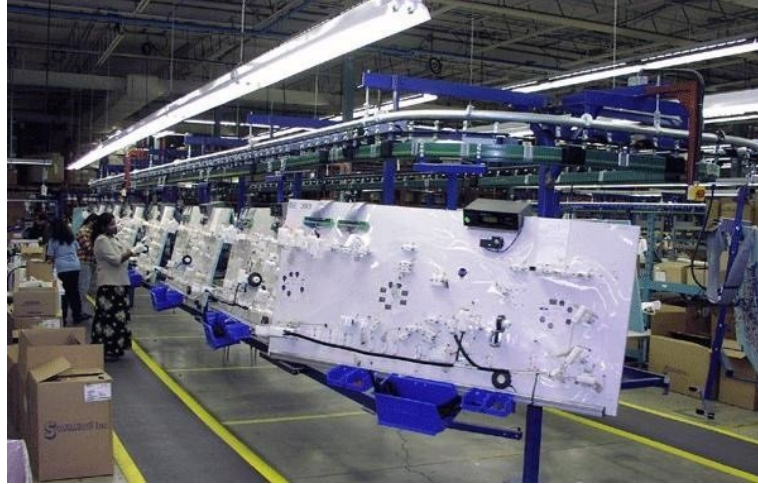
FIGURE C.1: A conveyor system of a wire harness assembly line, where parts, connectors, clips, and wires are placed on tables by operators [285]
