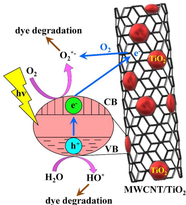
Figure 12. Mechanism of the photocatalytic degradation of dye with titanium dioxide-modified MWCNTs [162]
