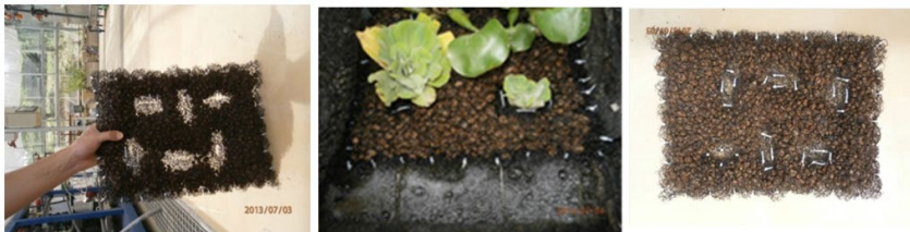
3.2.3. figure – Expanded clay cushion developed for FCR reactor aquatic plants
