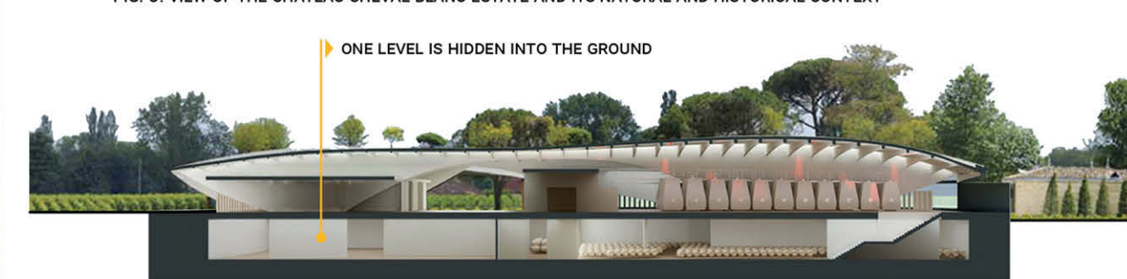
FIG. 10. CELLAR'S LONGITUDINAL SECTION, SHOWING THE CONNECTION WITH THE TERRAIN AND THE HOST BUILDINGS
