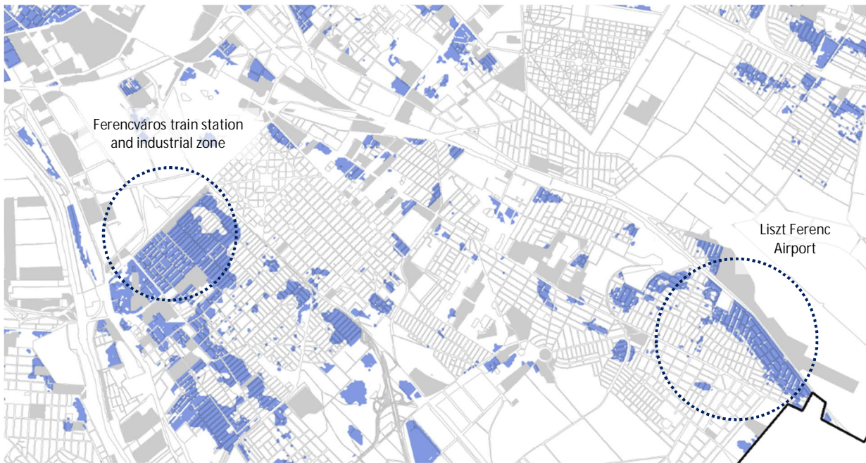
FIGURE 27: EVAPORATION APPLICABILITY MAP. EXAMPLES OF THE HEATING EFFECT IMPACT FROM INDUSTRIAL AREAS
