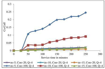
Fig.3.22 Effect of concentration 20, 100 mg L<sup>-1</sup>, flow rate 4ml/min, different bed heights (Felgyő compost, Cd<sup>2+</sup> treated)
