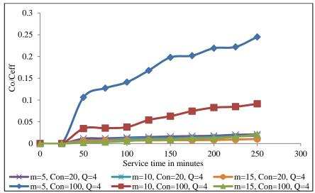
Fig. 3.28 Effect of concentration 20, 100 mg L<sup>-1</sup>, flow rate 4 ml/min, different bed heights (Felgyő compost, Cd<sup>2+</sup> treated)
