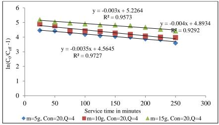
Fig. 3.62 Thomas plot of (Felgyő compost,  $Cd^{2+}$  treated) concentration 20 mg  $L^{-1}$  and 4 mL min<sup>-1</sup> flow rate and different bed heights
