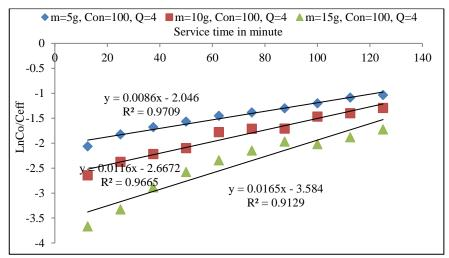
Fig. 3.49 Adams–Bohart plot of Felgyő compost, Cu<sup>2+</sup> concentration 100 mg L<sup>-1</sup> and 4 mL min<sup>-1</sup> flow rate and different bed heights
