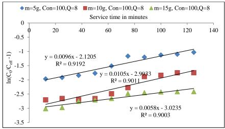
Fig. 3.57 Thomas plot (Garé compost, Cu<sup>2+</sup> treated) concentration 100 mg L<sup>-1</sup> and 4 mL min<sup>-1</sup> flow rate and different bed heights
