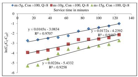
Fig. 3.77 Yoon–Nelson plot of (Felgyő compost, Cd<sup>2+</sup> treated) concentration 20 mg L<sup>-1</sup> and 4 mL min<sup>-1</sup> flow rate and different bed heights
