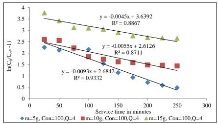
Fig. 3.60 Thomas plot of Felgyő compost, Cu<sup>2</sup> concentration 100 mg L<sup>-1</sup> and 4 mL min<sup>-1</sup> flow rate and different bed heights
