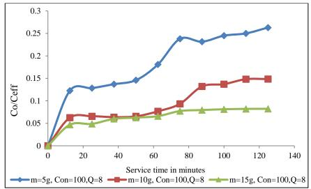
Fig. 3.33 Effect of bed height (Garé compost, Cu<sup>2+</sup> treated) at concentration 100 mg L<sup>-1</sup> and 8 mL min<sup>-1</sup> flow rate
