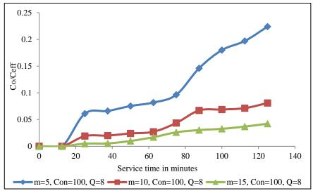
Fig. 3.41 Effect of bed height when concentration 100 mg L<sup>-1</sup> and flow rate 8 mL min<sup>-1</sup>. (Felgyő compost, Cd<sup>2+</sup> treated)
