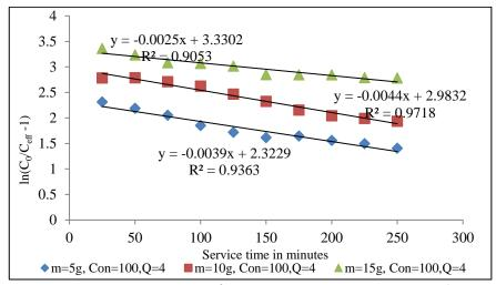
Fig. 3.56 Thomas plot (Garé compost,  $Cu^{2+}$  treated) concentration 100 mg  $L^{-1}$  and 4 mL min<sup>-1</sup> flow rate and different bed heights
