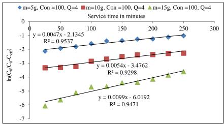
Fig. 3.76 Yoon–Nelson plot of (Felgyő compost,  $Cd^{2+}$  treated) concentration 20 mg  $L^{-1}$  and 4 mL min<sup>-1</sup> flow rate and different bed heights
