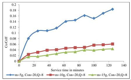
Fig. 3.31 Effect of bed height (Garé compost, Cu<sup>2+</sup> treated) at concentration 20 mg L<sup>-1</sup> and 8 mL min<sup>-1</sup> flow rate
