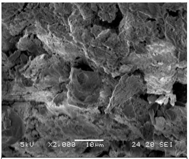
Fig. 3.3 Scanning electron microscopy (SEM) for Felgyő compost loaded with  $\text{Cu}^{2^+}$  at 10  $\mu m$
