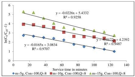
Fig. 3.65 Thomas plot of (Felgyő compost, Cd<sup>2+</sup> treated) concentration 20 mg L<sup>-1</sup> and 4 mL min<sup>-1</sup> flow rate and different bed heights
