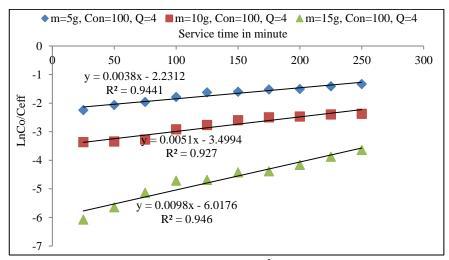
Fig. 3.52 Bohart–Adams plot of (Felgyő compost, Cd<sup>2+</sup> treated) concentration 20 mg L<sup>-1</sup> and 4 mL min<sup>-1</sup> flow rate and different bed heights
