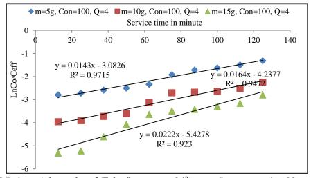
Fig. 3.53 Bohart–Adams plot of (Felgyő compost,  $Cd^{2+}$  treated) concentration 20 mg  $L^{-1}$  and 4 mL min<sup>-1</sup> flow rate and different bed heights
