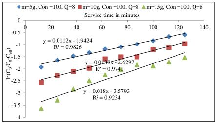
Fig. 3.73 Yoon–Nelson plot (Felgyő compost, Cu<sup>2+</sup> treated) Cu<sup>2+</sup> concentration 100 mg L-1 and 4 mL min-1 flow rate and different bed heights
