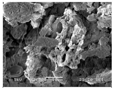
Fig. 3.7 Scanning electron microscopy (SEM) for Garé compost loaded with  $Cd^{2+}$  at  $10~\mu m$
