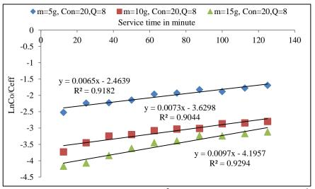
Fig. 3.43 Adams–Bohart plot (Garé compost, Cu<sup>2+</sup> treated) concentration 20 mg L<sup>-1</sup> and 8 mL min<sup>-1</sup> flow rate and different bed heights
