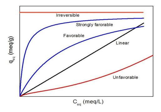
Fig. 2.2 Adsorption general isotherm curves
