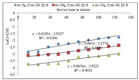
Fig. 3.47 Adams–Bohart plot of Felgyő compost, Cu<sup>2+</sup> concentration 20 mg L<sup>-1</sup> and 8 mL min<sup>-1</sup> flow rate and different bed heights
