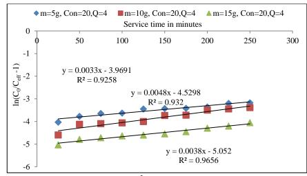
Fig. 3.54 Thomas plot (Garé compost,  $Cu^{2+}$  treated) concentration 20 mg  $L^{-1}$  and 4 mL min<sup>-1</sup> flow rate and different bed heights
