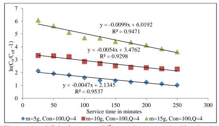
Fig. 3.64 Thomas plot of (Felgyő compost, Cd<sup>2+</sup> treated) concentration 20mg/l and 4 mL min<sup>-1</sup> flow rate and different bed heights
