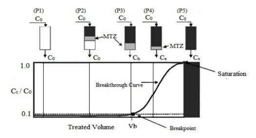
Fig. 2.4 (MTZ: mass transfer zone). Typical breakthrough curve for activated carbon showing the movement of the mass transfer zone according to the throughput volume
