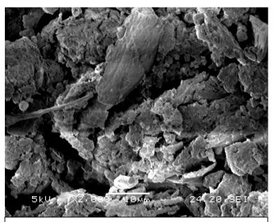
Fig. 3.6 Scanning electron microscopy (SEM) for Garé compost loaded with  $\text{Cu}^{2+}$  at 10  $\mu m$
