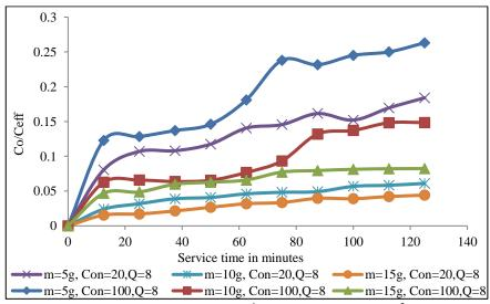
Fig. 3.19 Effect of concentration 20, 100 mg L<sup>-1</sup> at (Garé compost, Cu<sup>2+</sup> treated) different bed heights, flow rate 8 mL min<sup>-1</sup>
