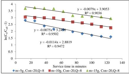
Fig. 3.59 Thomas plot of Felgyő compost, Cu<sup>2+</sup> concentration 20 mg L<sup>-1</sup> and 8 mL min<sup>-1</sup> flow rate and different bed heights
