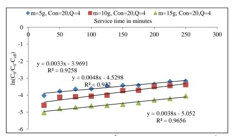
Fig. 3.66 Yoon–Nelson plot (Garé compost,  $Cu^{2+}$  treated) concentration 20 mg  $L^{-1}$  and 4 mL min<sup>-1</sup> flow rate and different bed heights
