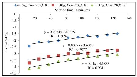
Fig. 3.67 Yoon–Nelson plot (Garé compost, Cu<sup>2+</sup> treated) concentration 20 mg L<sup>-1</sup> and 8 mL min<sup>-1</sup> flow rate and different bed heights
