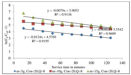
Fig. 3.63 Thomas plot of (Felgyő compost, Cd<sup>2+</sup> treated) concentration 20 mg L<sup>-1</sup>and 4 mL min<sup>-1</sup> flow rate and different bed heights
