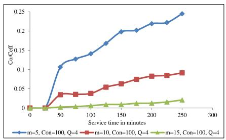
Fig. 3.40 Effect of bed height when concentration 100 mg L<sup>-1</sup> and flow rate 4 mL min<sup>-1</sup>
