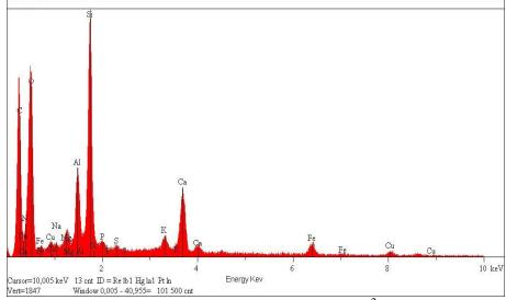
Fig. 3.9 Energy dispersive X-ray spectroscopy (EDX) after Cu<sup>2+</sup> loaded (Felgyő compost)
