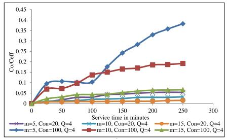
Fig. 3.20 Effect of concentration 20, 100 mg L<sup>-1</sup> at different bed heights, flow rate 4 mL min<sup>-1</sup> (Felgyő compost, Cu<sup>2+</sup> adsorbed)
