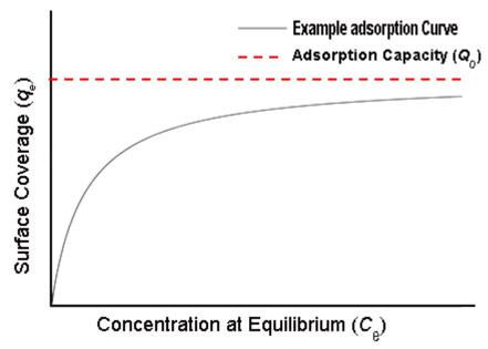
Fig. 2.1 Example adsorption isotherm
