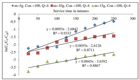
Fig. 3.72 Yoon—Nelson plot (Felgyő compost,  $Cu^{2+}$  treated)  $Cu^{2+}$  concentration 100 mg  $L^{-1}$  and 4 mL min<sup>-1</sup> flow rate and different bed heights
