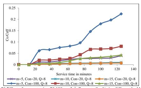
Fig. 3.29 Effect of concentration 20,100 mg L<sup>-1</sup>, flow rate 8 ml/min, different bed heights. (Felgyő compost, Cd<sup>2+</sup> treated)
