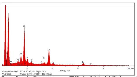
Fig. 3.13 Energy dispersive X-ray spectroscopy (EDX) after Cd<sup>2+</sup> loaded (Garé compost)
