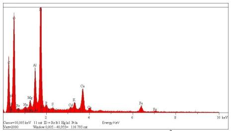
Fig. 3.10 Energy dispersive X-ray spectroscopy (EDX) after Cd<sup>2+</sup> loaded (Felgyő compost)
