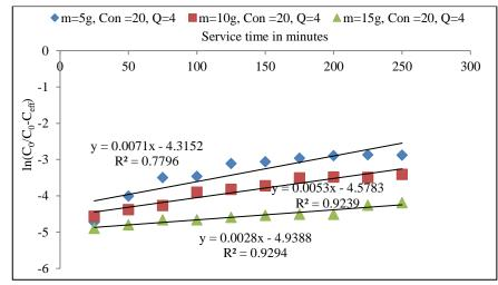
Fig. 3.70 Yoon–Nelson plot of Yoon–Nelson plot (Felgyő compost, Cu<sup>2+</sup> treated) Cu<sup>2+</sup> concentration 20 mg L<sup>-1</sup> and 4 mL min<sup>-1</sup> flow rate and different bed heights
