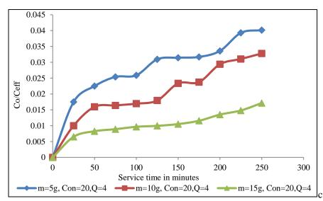
Fig. 3.30 Effect of bed height (Garé compost, Cu<sup>2+</sup> treated) at concentration 20 mg L<sup>-1</sup> and 4 mL min-<sup>1</sup> flow rate
