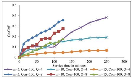
Fig. 3.27 Effect of the flow rate at 100 mg L<sup>-1</sup> Cu<sup>2+</sup> concentration at different bed heights, flow rate 4 mL min<sup>-1</sup> and (b) 8 mL min<sup>-1</sup> (Felgyő compost, Cu<sup>2+</sup> adsorbed)
