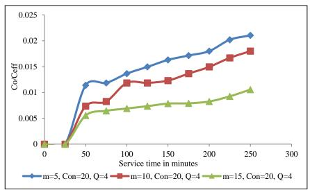
Fig.3.38 Effect of bed height when concentration 20 mg L<sup>-1</sup>and flow rate 4 mL min<sup>-1</sup>. (Felgyő compost, Cd<sup>2+</sup> treated)
