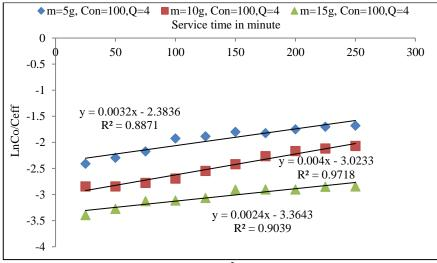
Fig. 3.44 Adams–Bohart plot (Garé compost, Cu<sup>2+</sup> treated) concentration 100 mg L<sup>-1</sup> and 4 mL min<sup>-1</sup> flow rate and different bed heights
