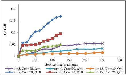
Fig. 3.26 Effect of the flow rate at 20 mg L<sup>-1</sup> Cu<sup>2+</sup> concentration at different bed heights, flow rate 4 mL min<sup>-1</sup> and 8 mL min<sup>-1</sup>, (Felgyő compost, Cu<sup>2+</sup> adsorbed)
