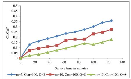
Fig. 3.37 Effect of bed height at concentration 100 mg L-1 and 8 mL min<sup>-1</sup> flow rate (Felgyő compost, Cu<sup>2+</sup> adsorbed)
