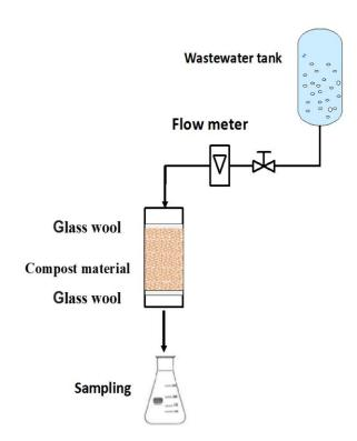
Fig. 3.1 Column experimental set up
