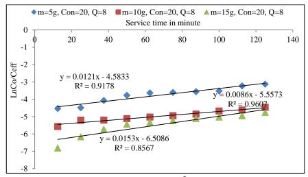
Fig. 3.51 Bohart–Adams plot of (Felgyő compost, Cd²+ treated) concentration 20 mg L¹-and 8 mL min¹-l flow rate and different bed heights
