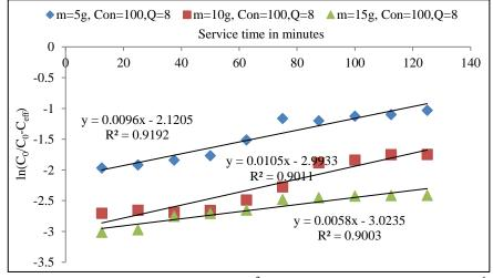
Fig. 3.69 Yoon–Nelson plot (Garé compost, Cu<sup>2+</sup> treated) concentration 100 mg L<sup>-1</sup> and 4 mL min<sup>-1</sup> flow rate and different bed heights
