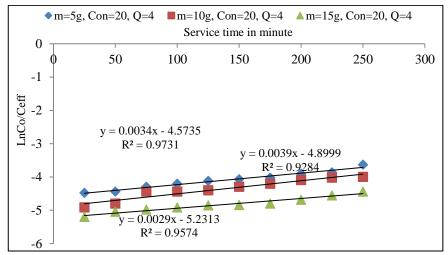
Fig. 3.50 Bohart–Adams plot of Felgyő compost,  $Cd^{2+}$  treated concentration 20 mg  $L^{-1}$  and 4 mL min<sup>-1</sup> flow rate and different bed heights
