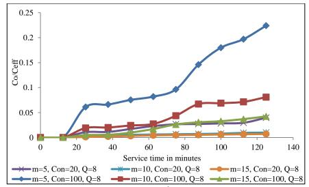
Fig. 3.23 Effect of concentration 20, 100 mg L<sup>-1</sup>, flow rate 8ml/min, different bed heights (Felgyő compost, Cd<sup>2+</sup> treated)
