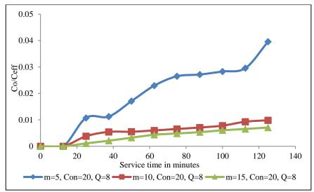
Fig. 3.39 Effect of bed height when concentration 20 mg L<sup>-1</sup> and flow rate 8 mL min<sup>-1</sup>. (Felgyő compost, Cd<sup>2+</sup> treated)
