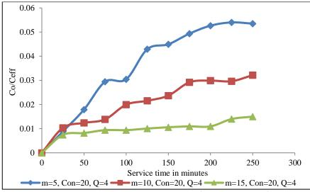
Fig. 3.34 Effect of bed height at concentration 20 mg L<sup>-1</sup> and 4 mL min<sup>-1</sup> flow rate, (Felgyő compost, Cu<sup>2+</sup> adsorbed)
