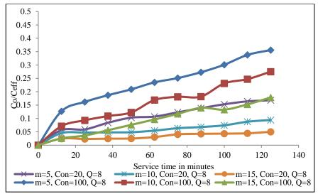
Fig. 3.21 Effect of concentration 20, 100 mg L<sup>-1</sup> at different bed heights, flow rate 8 mL min<sup>-1</sup> (Felgyő compost, Cu<sup>2+</sup> adsorbed)
