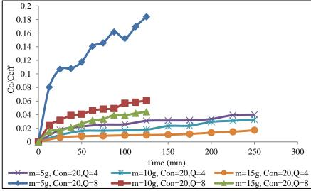
Fig. 3.24 Effect of flow rate (Garé compost, Cu<sup>2+</sup> treated) at 20 mg L<sup>-1</sup> concentration at different bed heights, flow rate 4 and 8 mL min<sup>-1</sup>
