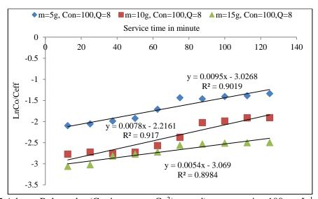
Fig. 3.45 Adams–Bohart plot (Garé compost, Cu<sup>2+</sup> treated) concentration 100 mg L<sup>-1</sup> and 4 mL min<sup>-1</sup> flow rate and different bed heights
