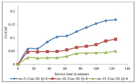
Fig. 3.35 Effect of bed height at concentration 20 mg L<sup>-1</sup> and 4 mL min<sup>-1</sup> flow rate (Felgyő compost, Cu<sup>2+</sup> adsorbed)
