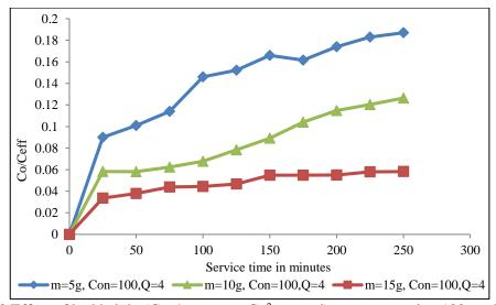
Fig. 3.32 Effect of bed height (Garé compost, Cu<sup>2+</sup> treated) at concentration 100 mg L<sup>-1</sup> and 4 mL min<sup>-1</sup> flow rate
