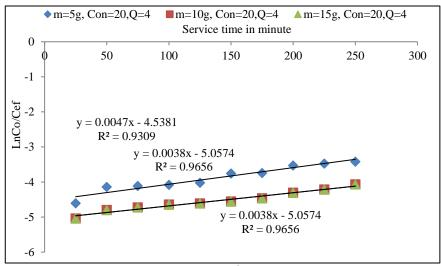
Fig. 3.42 Adams–Bohart plot (Garé compost, Cu<sup>2+</sup> treated) concentration 20 mg L<sup>-1</sup> and 4 mL min<sup>-1</sup> flow rate and different bed heights
