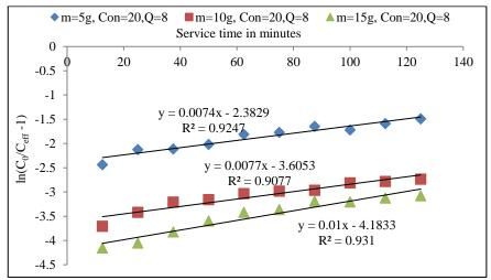
Fig. 3.55 Thomas plot (Garé compost, Cu<sup>2+</sup> treated) concentration 20 mg L<sup>-1</sup> and 8 mL min<sup>-1</sup> flow rate and different bed heights
