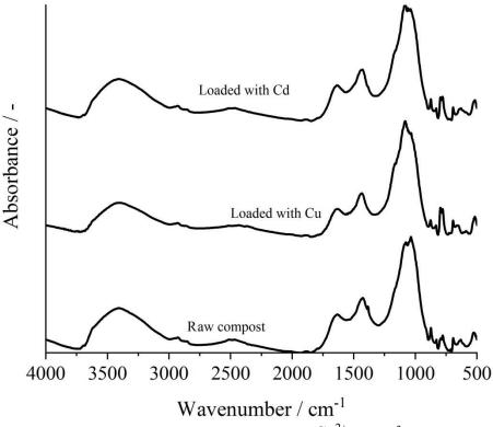
Fig. 3.15 FTIR spectra of raw Felgyő compost loaded with  $Cu^{2+}$  and  $Cd^{2+}$ .
