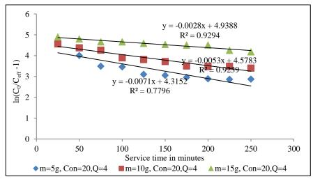
Fig. 3.58 Thomas plot of Felgyő compost, Cu<sup>2+</sup> concentration 20 mg L<sup>-1</sup> and 4 mL min<sup>-1</sup> flow rate and different bed heights
