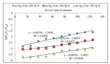
Fig. 3.71 Yoon–Nelson plot (Felgyő compost,  $Cu^{2+}$  treated)  $Cu^{2+}$  concentration 20 mg  $L^{-1}$  and 8 mL min<sup>-1</sup> flow rate and different bed heights
