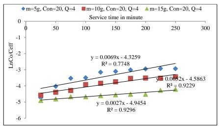
Fig. 3.46 Adams–Bohart plot of Felgyő compost, Cu<sup>2+</sup> concentration 20 mg L<sup>-1</sup> and 4 mL min<sup>-1</sup> flow rate and different bed heights
