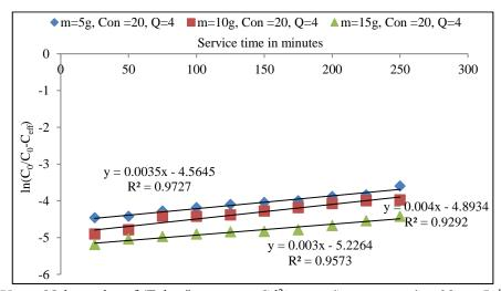
Fig. 3.74 Yoon–Nelson plot of (Felgyő compost,  $Cd^{2+}$  treated) concentration 20 mg  $L^{-1}$  and 4 mL min<sup>-1</sup> flow rate and different bed heights
