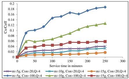
Fig. 3.18 Effect of concentration 20, 100 mg L-1 at (Garé compost, Cu<sup>2+</sup> treated) different bed heights, flow rate 4 mL min<sup>-1</sup>
