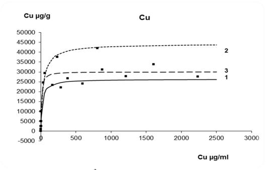
Fig. 3.16 Experimental data of  $Cu^{2+}$ adsorbed by compost (Sioagárd, Garé and Felgyő) fitted to Langmuir model
