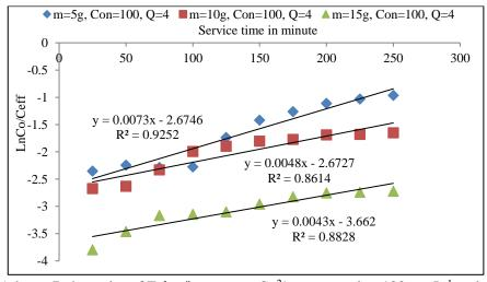
Fig. 3.48 Adams–Bohart plot of Felgyő compost,  $Cu^{2+}$  concentration 100 mg  $L^{-1}$  and 4 mL min<sup>-1</sup> flow rate and different bed heights
