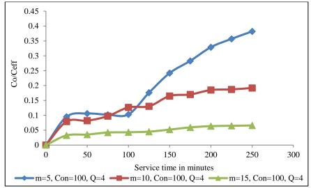
Fig. 3.36 Effect of bed height at concentration 100 mg L<sup>-1</sup> and 4 mL min<sup>-1</sup> flow rate (Felgyő compost, Cu<sup>2+</sup> adsorbed)
