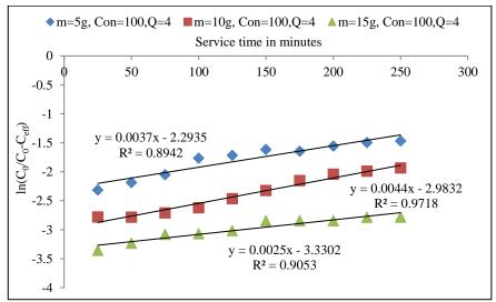
Fig. 3.68 Yoon–Nelson plot (Garé compost, Cu<sup>2+</sup> treated) concentration 100 mg L<sup>-1</sup> and 4 mL min<sup>-1</sup> flow rate and different bed heights
