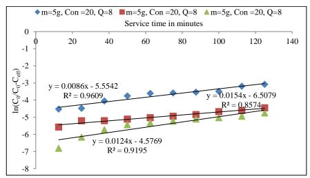
Fig. 3.75 Yoon–Nelson plot of (Felgyő compost,  $Cd^{2+}$  treated) concentration 20 mg  $L^{-1}$  and 4 mL min<sup>-1</sup> flow rate and different bed heights
