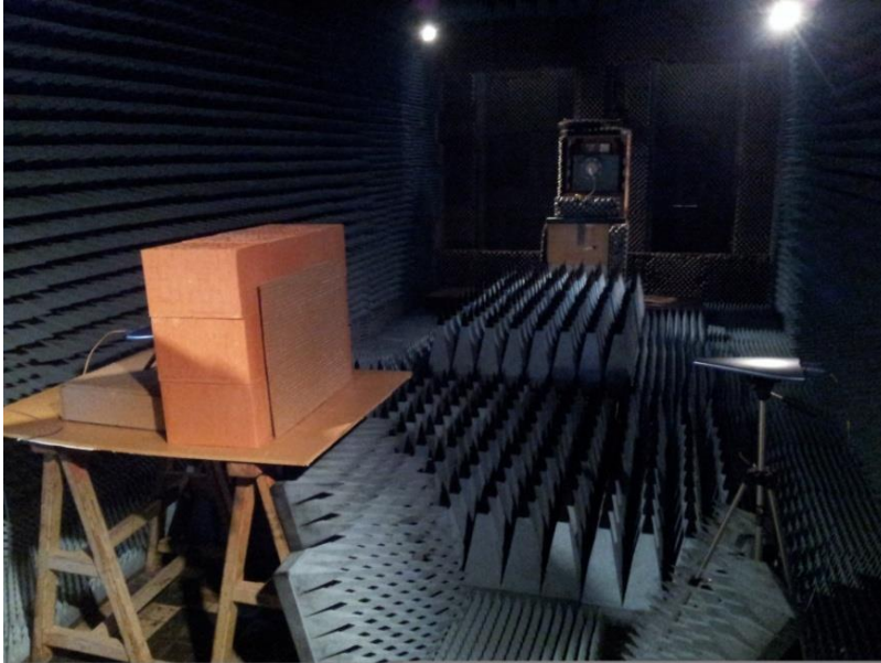
Fig 2. The arrangement of the measurement in the anechoic chamber with two Hyperlog antennas
