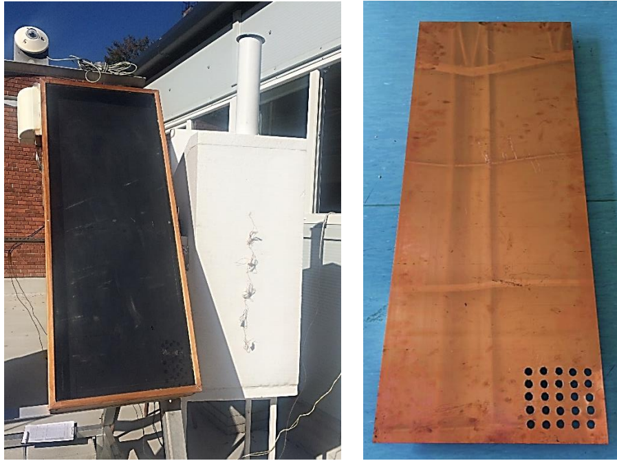
Fig. 4.9. Double-pass solar collector integrated with drying chamber and the un-finned absorbing surfaces
