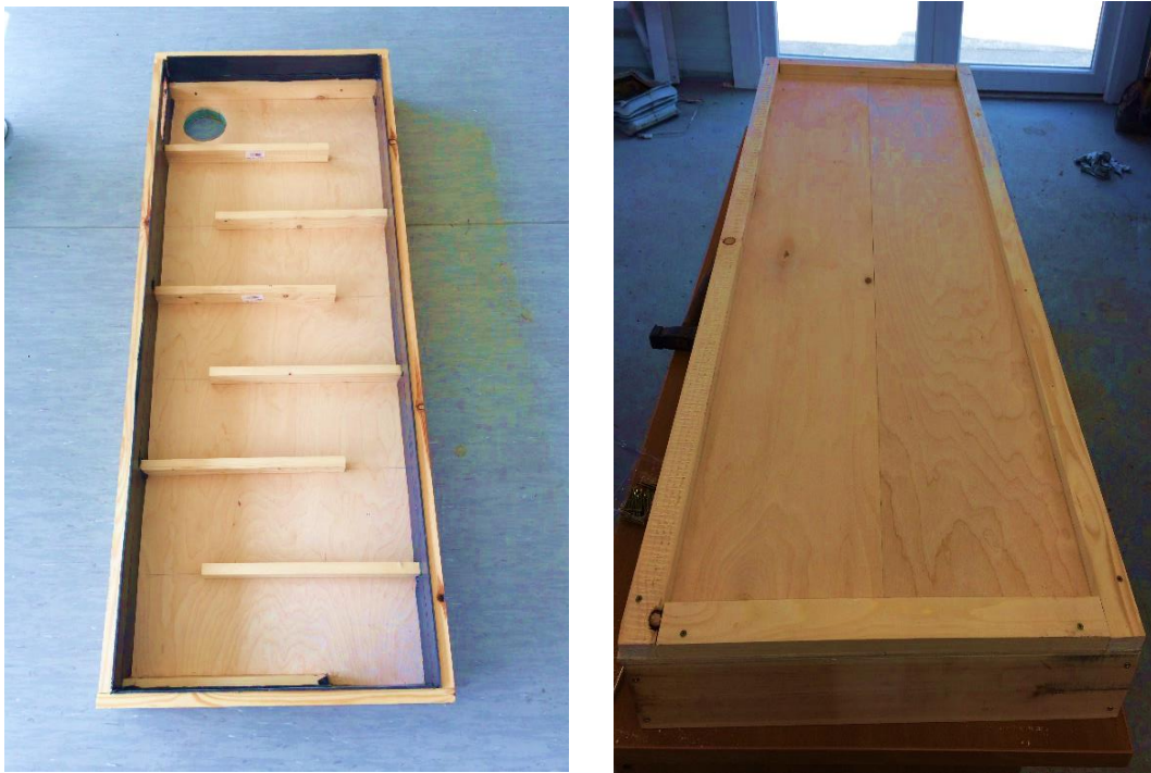
Fig. 3.15. First and second air pass of solar air heaters manufactured
