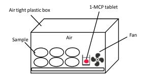
Figure 1. Schematic diagram of conventional 1-MCP application
