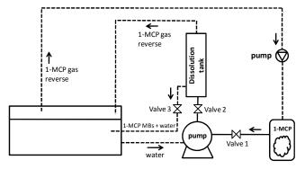
Figure 2. Schematic diagram of 1-MCP MBs generation system
