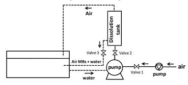
Figure 4. Schematic diagram of hot water and microbubbles generation system
