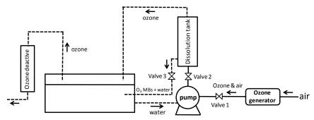
Figure 3. Schematic diagram of ozone microbubbles generation system
