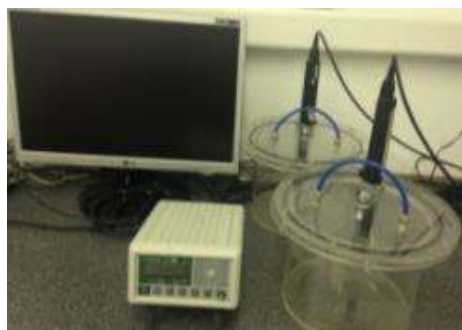
Figure 18. Respiration system containing the FY A600-CO 2 H carbon dioxide sensors connected to an Almemo 3290-8 data logger
