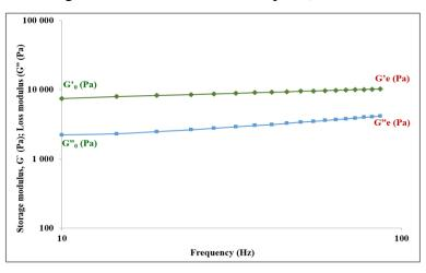
Figure 2. Frequency sweep rheogram and parameters
