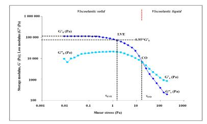
Figure 1. Amplitude sweep rheogram and parameters
