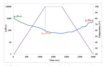
Figure 4. Heating temperature-dependent rheogram and parameters
