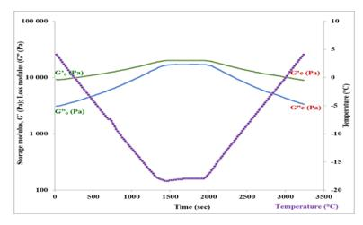
Figure. 3. Cooling temperature-dependant rheogram and parameters
