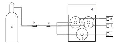
**Fig. 1.** Scheme of the developed flow-through apparatus: (a) compressed air, (b) activated charcoal filter, (c) HEPA filter, (d) thermostat, (e, f, g) sampling vials, and (h, i, j) portable carbon dioxide monitor
