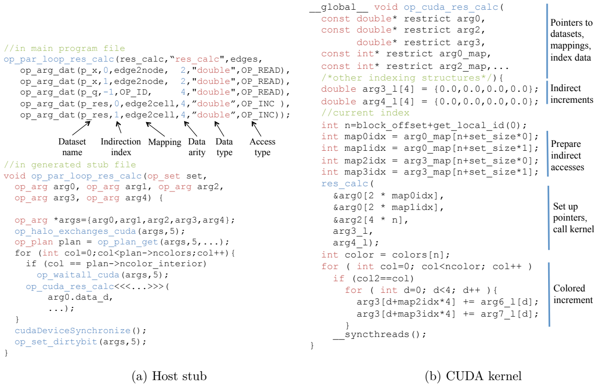
Figure 7.3. Code generated for execution on the GPU with CUDA
