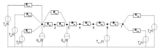
Fig. 9. The heat resistance model of a PV/T module (HR-PVT)
