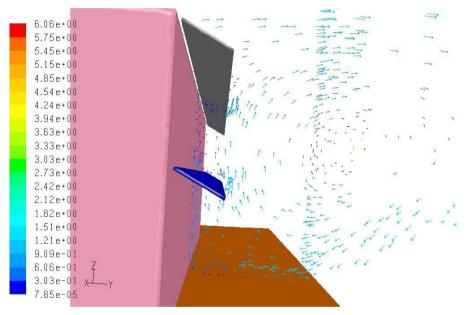
Fig. 4. The air flow vectors colored by the velocity in case of 3 m/s north wind
