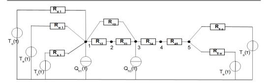
Fig. 6. The heat resistance model of a typical PV module
