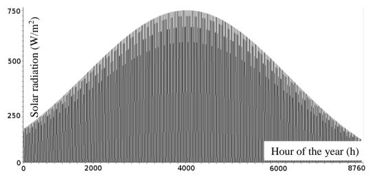
Fig. 1. Calculated chart of yearly solar radiation  $(W/m^2)$
