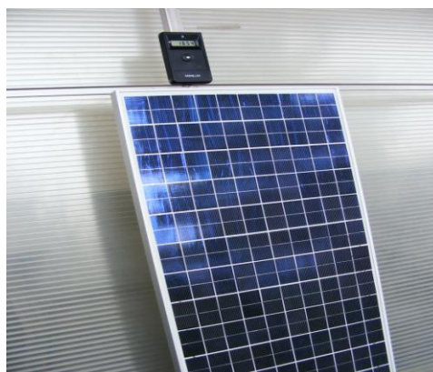
Fig. 3.13. Solar module with illuminance meter
