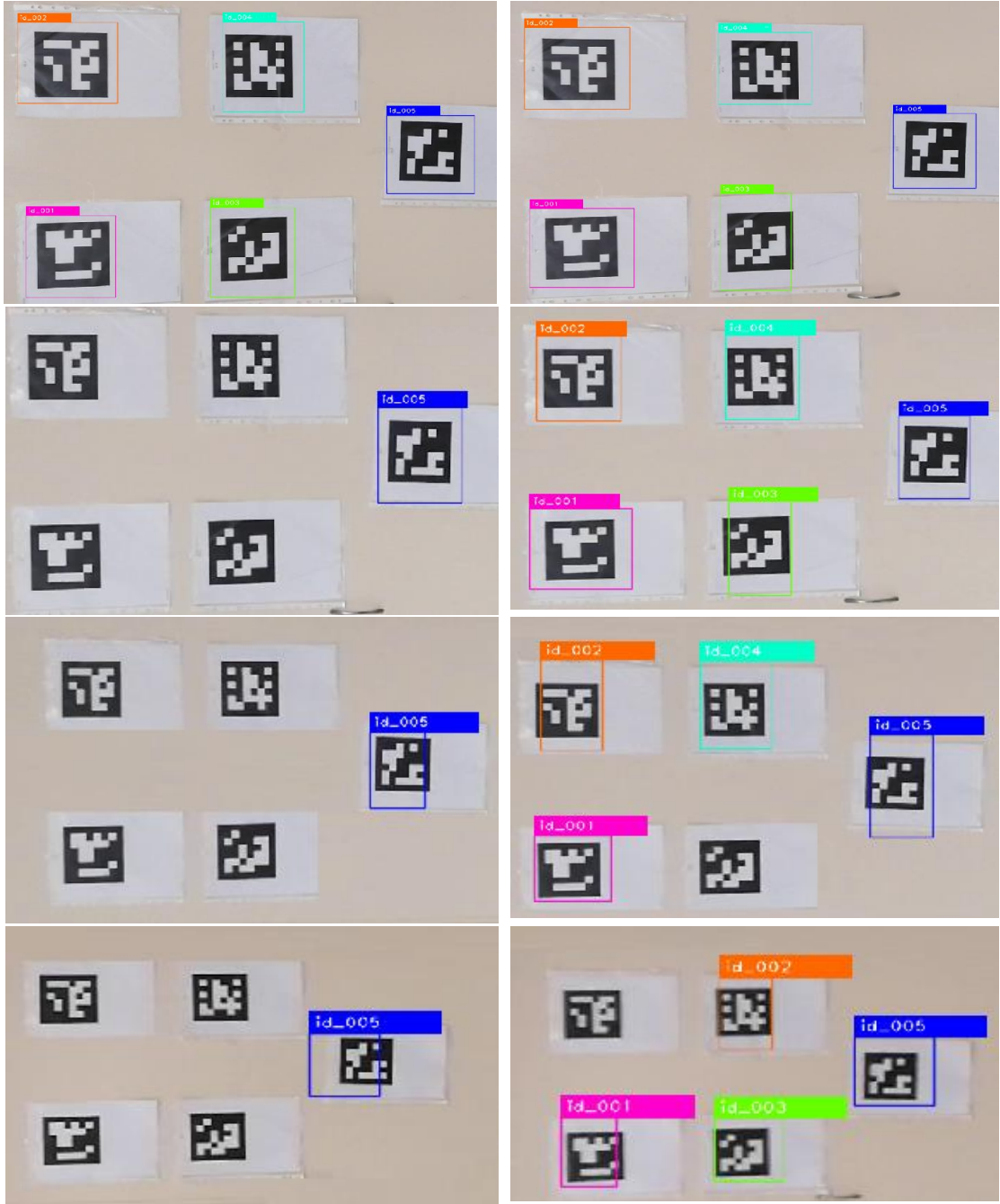
(a) Original version (b) Modified versions Figure 6-10. Screenshots of detected markers from different distances.
