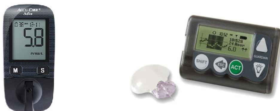
Figure 4. Ordinary fingertip blood glucose meter (left) and glucose monitoring with Continuous Glucose Monitoring device (right).
