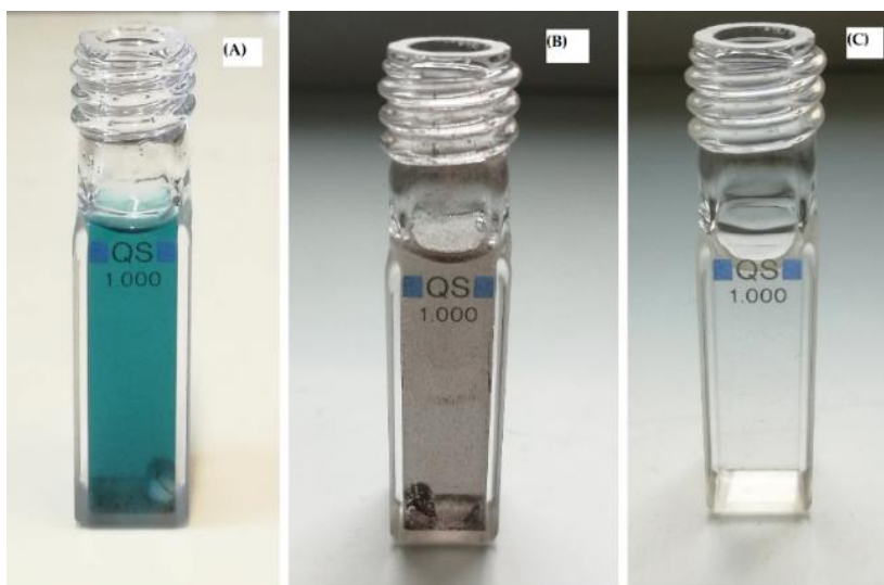
Figure 35. (A) Methylene blue spectrum, (B) UV/visible spectrum obtained after MB degradation using NP-3 ( \text{Cu}^{\text{II}}_{0.4}\text{Fe}^{\text{II}}_{0.6}\text{Fe}^{\text{III}}_2\text{O}_4 ), Concentrations: MB = 1.5 \times 10^{-5} mol/L, NPs = 400 mg/L, initial pH = 7.5, \text{H}_2\text{O}_2 = 1.76 \times 10^{-1} mol/L, temperature = 25 \pm 2 °C, and time = 140 min.
