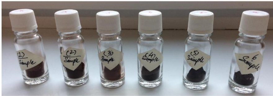
Figure 9. Dark powdered catalysts obtained after calcination process as results of co-precipitation and calcination process
